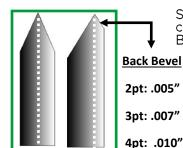
Support back bevels must be considered when using Side Bevel rule.
