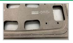
Extra bridges help maintain the correct cut size. Bridges add strength to the die and help keep long spans straight.
